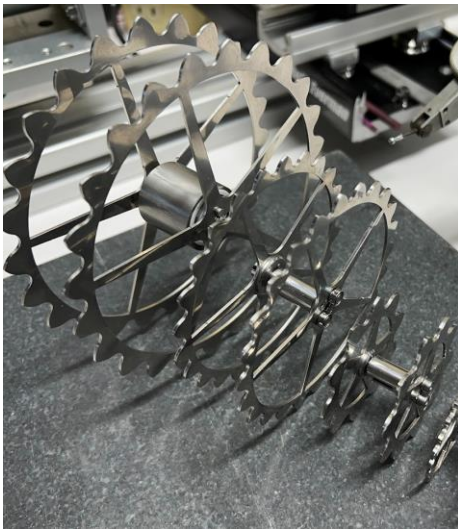
Figure 6. Wheel sets on their arbor bearing cartridges
