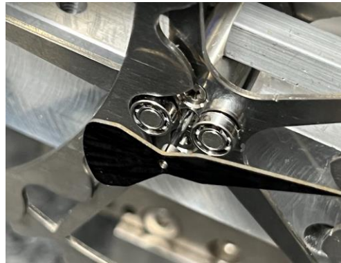
Figure 7. One side of the two-tooth pinion
