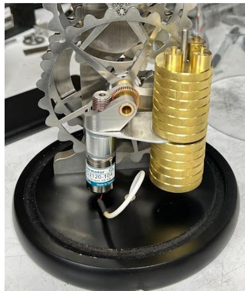
Figure 8. Worm drive rewriter
