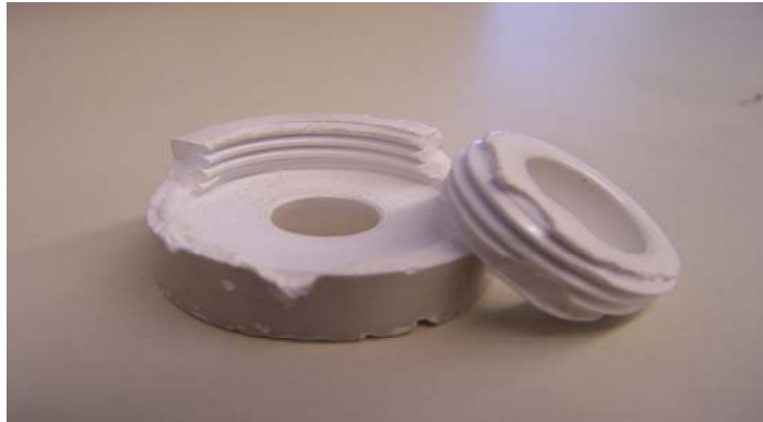
Figure 13. Failure of Existing Ceramic Insulator Threads
