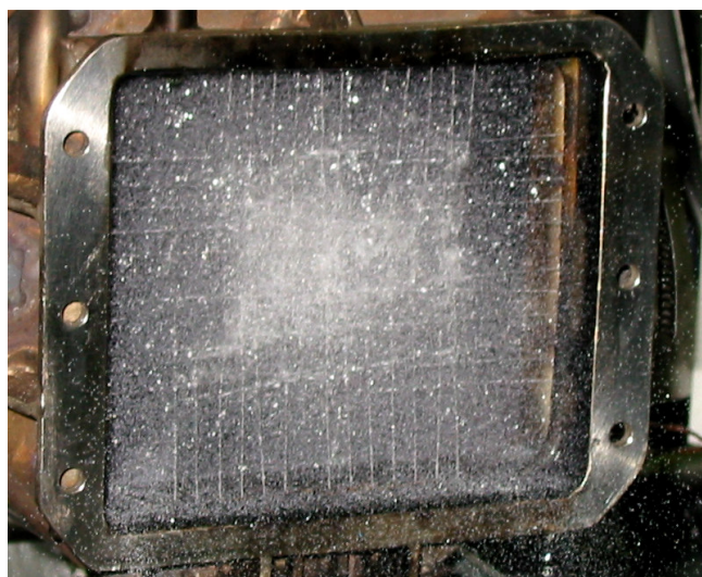
Figure 6. Flow Visualization of Pulsejet Fuel Injection
