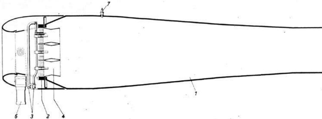
Fig. 1 – Diagram of the Argus engine of the Fiesseler (V-1) flying bomb
