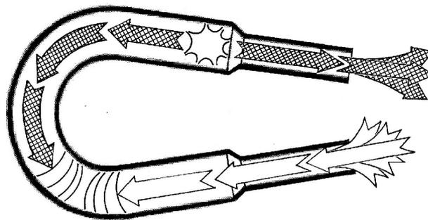
Fig. 11 – Expansion in the upper combustion chamber and intake in the lower
