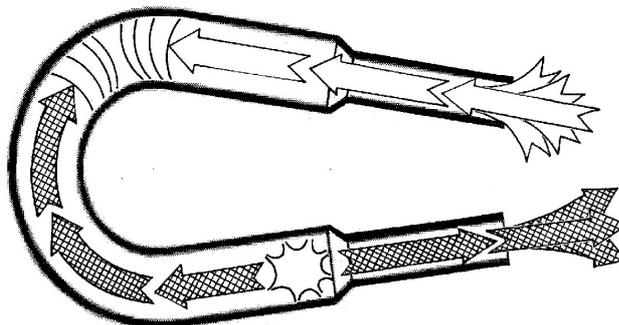
Fig. 13 – Expansion in the lower combustion chamber and intake in the upper
