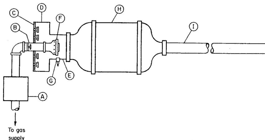
Fig. 3 – A simplified diagram of a Lennox Pulse burner for central heating
