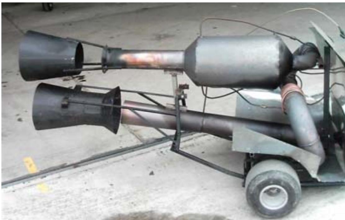
[As an aside -- the picture also shows the way a pulsejet can be bent. Unlike the steady-flow jet engines, pulsejets do not appear to be greatly affected by bends in their ducts. The reason is not quite clear. I think that the peculiar nature of the pulsejet flow -- part flow and part wave -- could be the reason. Unlike flows, waves are not bothered by turns and can
