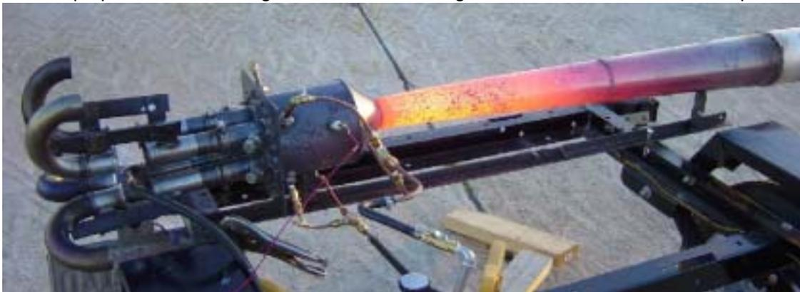
very short straight engine with four intake pipes. The intakes and the exhaust were adjustable for length to allow variations in the testing program.
