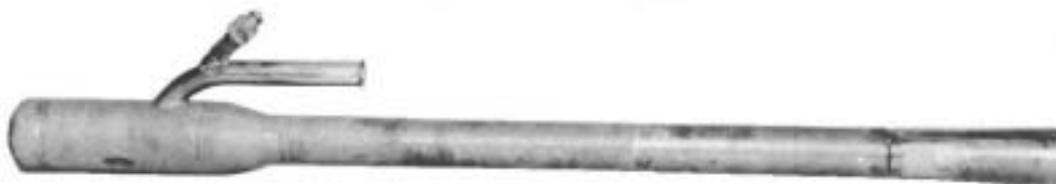
The NRL report made the rounds and apparently impressed somebody at the Low Temperature Laboratory at the National Research Council of Canada. Low temperature research is not easily associated with pulsejets, but that is what happened. Taking a good look at the NRL engine, the guys in Canada developed the above 3'6" machine that developed 3.5 lbs thrust.
