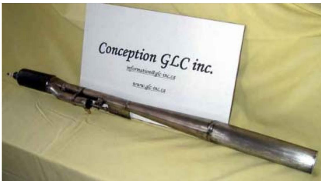
The engine is back in production, after a fashion. You can order stainless steel parts from Conception GLC Inc, a Canadian company run by pulsejet enthusiasts and involved in several interesting engine designs. The picture above shows the engine put together from their parts kit.
